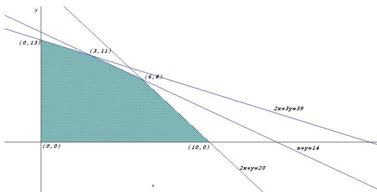
$$\begin{aligned} z(0, 13) &= 13000 \\ z(3, 11) &= 15500 \\ z(6, 8) &= 17000 \\ z(10, 0) &= 15000 \end{aligned}$$
